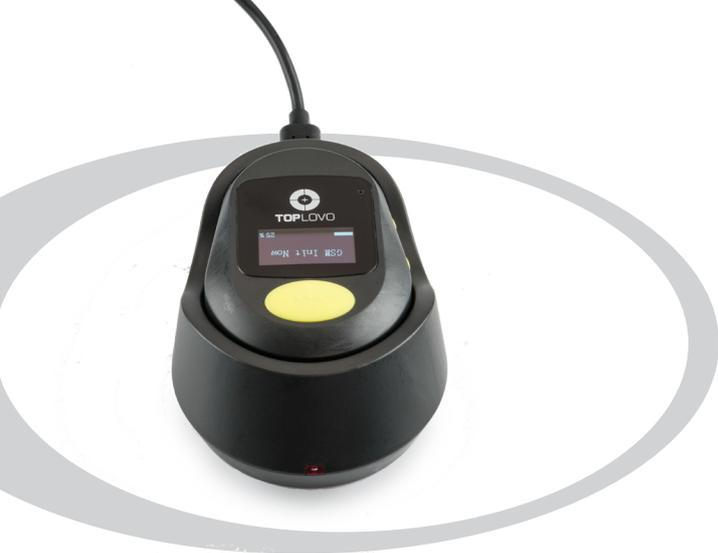
Make sure you have fully charged the pendant for around 2-3 hours before you begin to set up. You can either use the docking station supplied to charge the pendant or you can use the USB cord supplied to plug the pendant directly into your computer or car (if your car stereo has a USB connection) to charge it.
